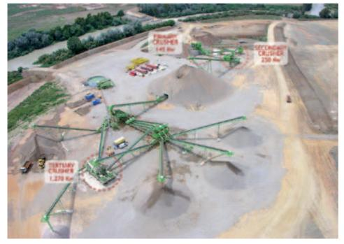
Figure 9. A crushing plant for quarried sand.
