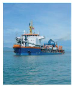
Figure 10. Trailer suction hopper dredger with  $10,000 \text{ m}^3$  capacity.
