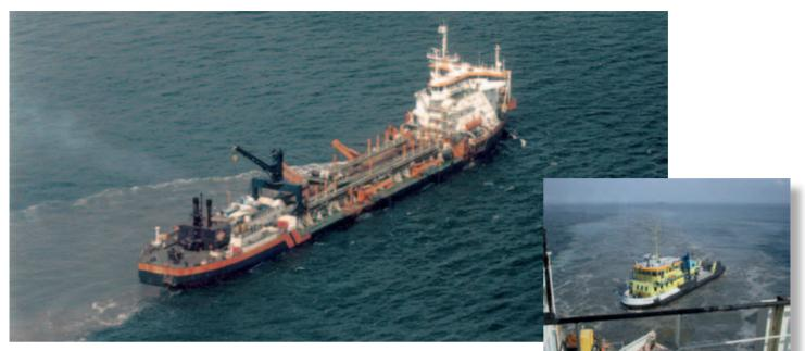
Figure 8. Short, limited extent of plume from a dredger (left), and plume being measured by a survey boat.
